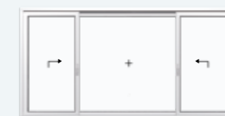
System K 2 lift/sliding sashes, 1 fixed pane
