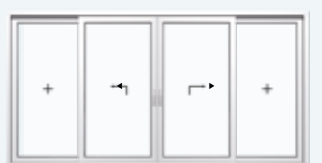
System C 2 lift/sliding sashes, 2 fixed panes
